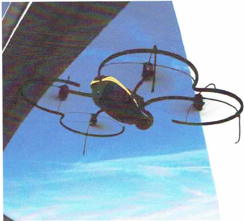
The SenseFly Exom is billed as the intelligent mapping and inspection drone designed to fly an autonomous, GPS-guided mission. Its "ScreenFly" feature observes structures and surfaces live, in real time.
